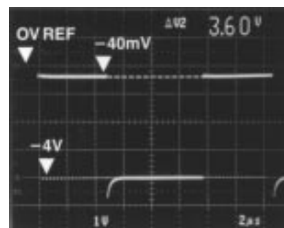
Figure 3-14. Bias/Offset adjusted for -4 V. Signal current at the -4 V level is zero. Current flow at ground level is maximum (10% down).
